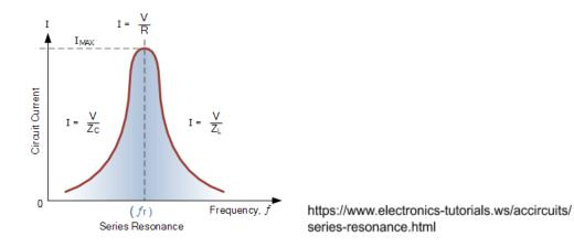
The peak in the middle corresponds to the **resonance frequency**, which is the frequency at which  $X_L$  and  $X_C$  are equal, and therefore, in this formula  $Z = \sqrt{(X_L - X_C)^2 + R^2}$ , they cancel each other out, leaving Z=R. Both reactances are functions of angular frequency, and thus an expression for the **resonant frequency** can be found:
