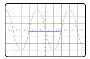
From the settings of the oscilloscope it can be determined how many V per division in the y axis, and seconds per division for the x axis are shown.
