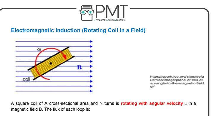
**Flux** =  $BA \cos\theta$ , where  $\theta$  is the angle between the magnetic field and the normal of the coil.
